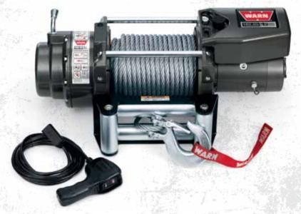
**16.5ti** Highest capacity, most technologically advanced winch for big trucks. Series-wound motor combined with a 3-stage planetary gear train delivers 16,500 lbs. of pulling power. Thermometric indicator LED provides operator feedback on motor temperature.
