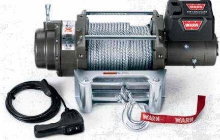
M12000 Champion workhorse for heavy-duty winching. 3-stage planetary geartrain combined with a 4.6hp series-wound motor produce 12,000 lbs. of pulling power. Design is low profile so it fits where you want it.
