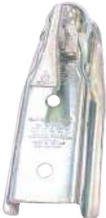
Fulton coupler after 336 hours salt spray testing.
