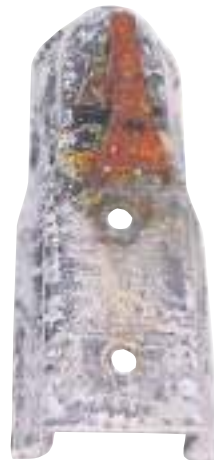
Competitor's coupler after 336 hours salt spray testing.
