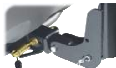
Secure ball mount or hitch-mounted accessory with locking head
