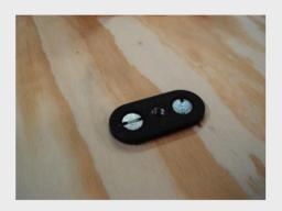
Now attach each plate using the 5/16" x 18tpi countersunk screws and locknuts and washers underneath.
