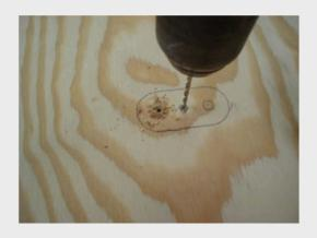
Now use a small drill bit to pilot drill the three hole locations under each mounting plate.
