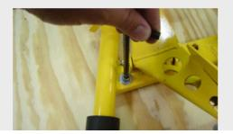
Now you will be able to quickly set your chock over the mounting plates and attach it using the 3/8"x 16tpi allen head bolts supplied with the kit.
