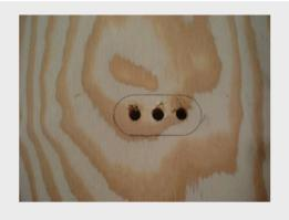
Now drill out the three holes using a 3/8" drill bit.
