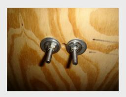
Spread the large washers apart from the center hole so they will not interfere with the chock mounting bolt.
