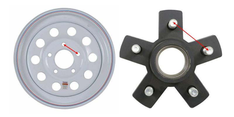
In order to determine the bolt pattern, measure the distance from the center of a stud to an adjacent stud as shown on the images above. If the center of stud to center of adjacent stud distance is:
