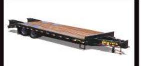
Pintle Equipment Transport Trailer available in 102" width and in lengths of 20' + 5' and 24' + 5' • Approximate Carrying Capacity ranges from 22,800# to 24,000#, depending on length • Integral Tongue with 12", 19# I-Beam Frame 60K, 3" ID Three Position Pintle Eye
