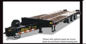
Pintle Heavy Equipment Transport Trailer available in 102" width and in lengths of 24' and 28' • Approximate Carrying Capacity ranges from 47,100# to 47,600#, depending on length • Integral Tongue with 14", 26# I-Beam Frame • 60K, 3" ID 3 Position Pintle Eye • 12K Top Wind Drop Leg Jack Low Profile Bed with Oak Flooring
